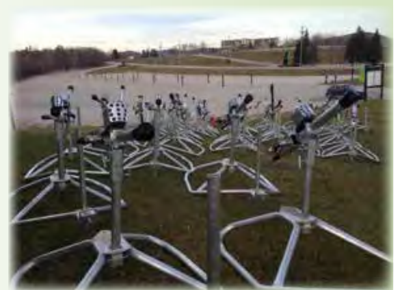
Shipment of high-efficiency Snow Logic snow guns awaiting installation at a Vermont ski area. Photos courtesy Efficiency Vermont.
