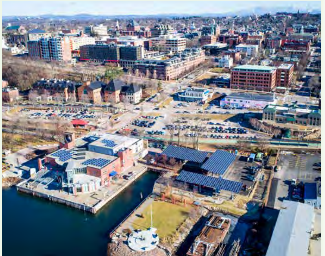
Vermont's largest parking lot solar canopy, a 156kW system, at the ECHO, Leahy Center for Lake Champlain. This is just part of what promises to be impressive work we will report on soon. Image courtesy of Encore Renewable Energy.
